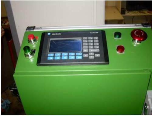
stop button (the operator cannot stop the test until at least ten minutes have passed). When the operator stops the test, the pressure reading at the end of test, the time of test, and pressure loss during the test are displayed on the operator interface. A red (fail) or a green (pass) indicator will also light and the unit being tested will depressurize. The operator can then either repair the unit or send it to be installed on the machine.
