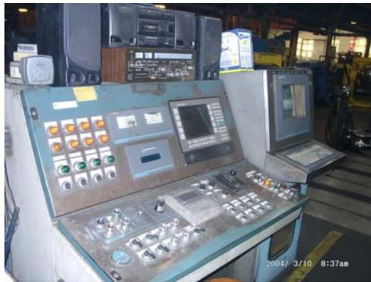
lengths. The controls included three Nematron industrial control computers, a main control computer in a cool room, and a Reliance DCS PLC. The computers were running an outdated version of Wonder Ware software and communicating with the DCS network through an Ethernet loop. Because of this loop, if any one of the
